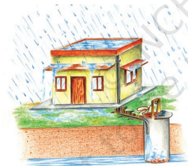
(b) Recharge through Abandoned Dugwell
